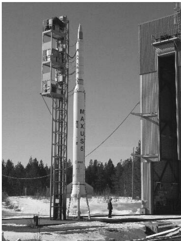
Fig. 4 Maxus rocket has an overall length of 15.8 m and a total mass of 11.4 tons. It employs a Morton Thiokol Castor 4B motor, which develops a thrust of 430 kN over a 64-s burn time.
