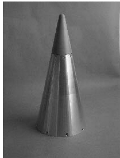
Fig. 2 Helical tip antenna with radome for GPS tracking of sounding rockets during the early flight phase (DLR Mobile Rocket Base).
